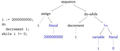
A program is an Abstract Syntax Tree data structure in memory: heap-allocated structs and unions with lots of pointers. Each node has an enum field to distinguish its kind.
